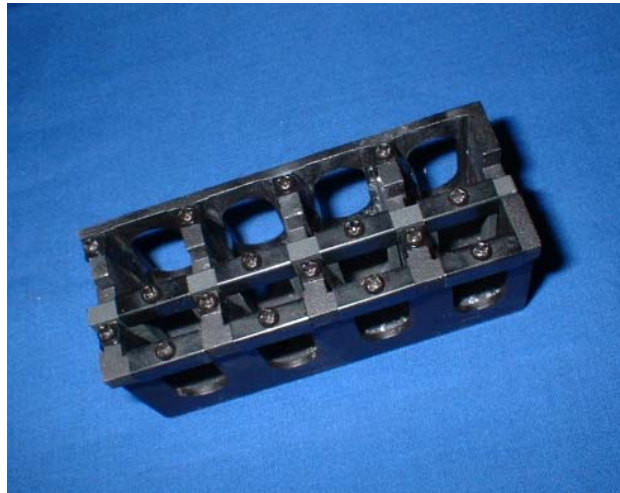
Fig. 1-3 Rectangular Standard Four Cell Holder for HALO RB-10 Accessory
