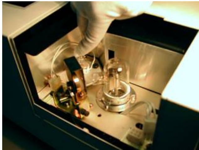
Fig. 5-4 Secure the WI lamp position
