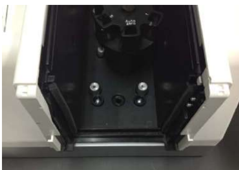
Fig. 5-101 Sample Compartment with the Cover Removed
