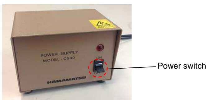
Fig. 5-99 Power Supply for the Pen-Type Low-Pressure Mercury Lamp
