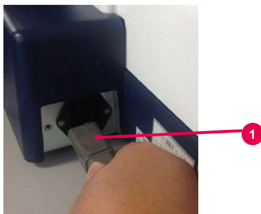
Fig. 7-14 Unplugging Power Cable
