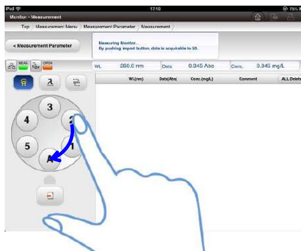
Fig. 2-18 Drag Operation (An Example of Moving Cell 2 to Measuring Position)
