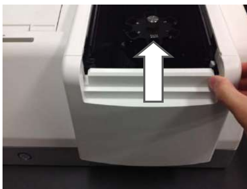
Fig. 5-100 Removing the Front Cover of the Sample Compartment
