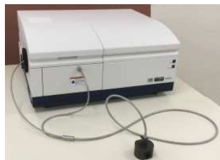
Model F-7100 Fluorescence Spectrophotometer (Optical fiber attachment installed)
