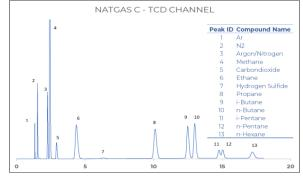
Figure 2: Permanent gases on TCD channel
