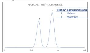
Figure 4: Helium and Hydrogen analysis on TCD channel
