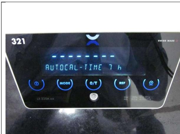
Long press "Mode" key to enter the AutoCal time. Short press "Mode" key to select the time. In this case, short press the first digit to "0" then long press the "Mode" key to move to 2<sup>nd</sup> digit. Short press "Mode" key to select 7 and the long press "Mode" key to confirm.
