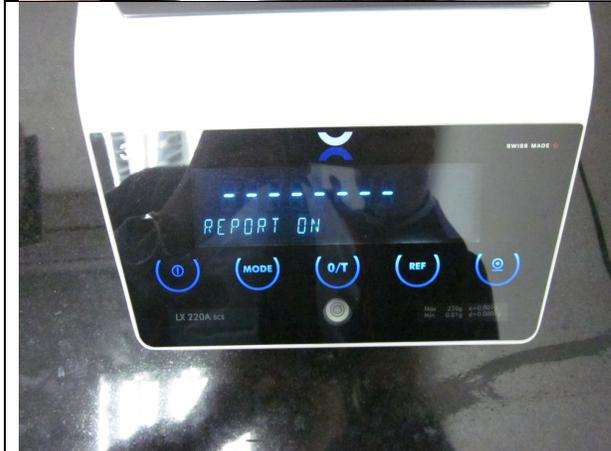
Long press "Mode" key to enter the Report mode. Short press "Mode" key to turn on the Report. After each auto calibration, it will display the result. . Long press "Mode" to confirm.
