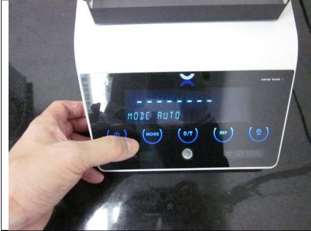
Release the "Mode" key. Then long press the "Mode" menu appears. Then short press the "Mode" key to select the Calibration mode to be Auto. Then long press the "Mode" key to confirm.
