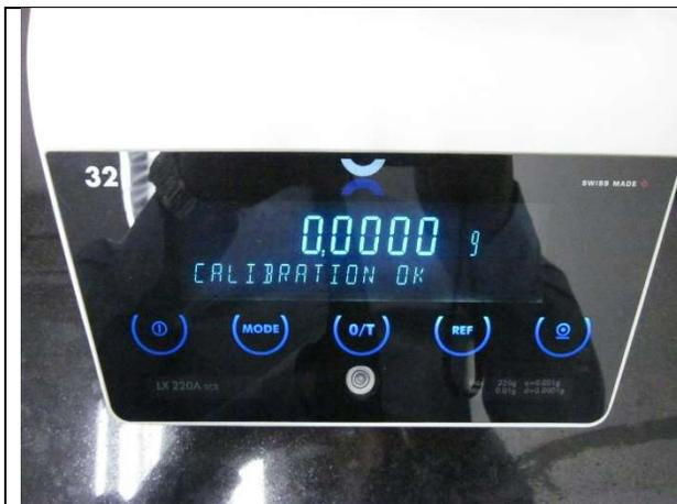
Calibration result is displayed after each auto calibration. In this case, it display calibration "OK".
