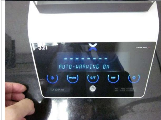
Long press "Mode" key to enter the Auto-warning. Short press "Mode" key to turn on the Auto warning. When temperature is out of range, it will prompt the user to perform the calibration. Long press "Mode" to confirm.
