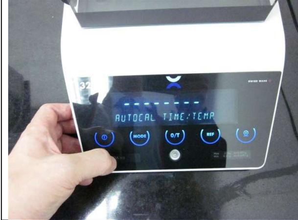
Long press the "Mode" key to enter the Autocal mode: Short press the "Mode" key to select Time/Temp or Time. Long press the "Mode" key to confirm.
