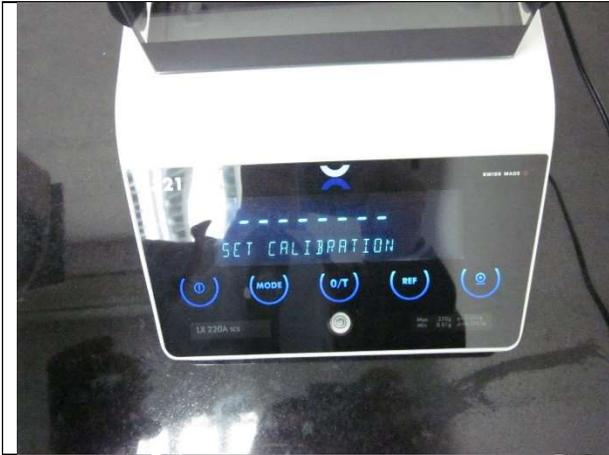
Press the "Mode" continuously until "Set Calibration" menu appears.
