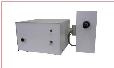
Substandard light source
