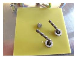
Lay the plate (340-7216) like in the picture on the heating plate and tight the screw (PN1100-104, M4x8)
