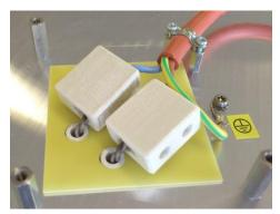
Assemble the three wires by using the two clamps (3950-161) and one screw (1100-172, M4x12 and two washers PN 1500-027).
