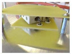
Lay the plate (340-7217) with three holes in the corner on the bolts and assemble it with the screws (1100-211, M4x6)
