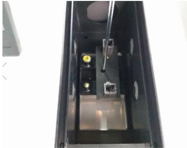
Figure 4-2 Screw/Unscrew the screw of cuvette holder
