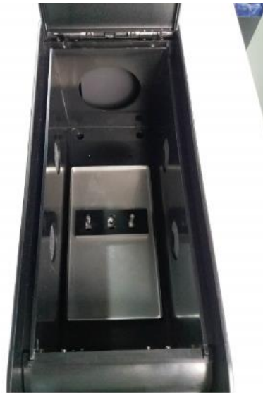
Figure 4-3 Remove/mount cuvette holder
