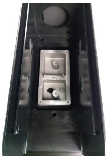
Figure 4-4 Sample chamber after removing cuvette holder
