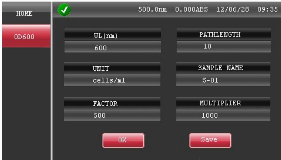
When select UNIT cells/ml, it will display above parameter setting interface
