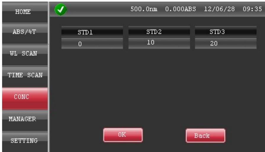
If using standard sample regression calculation method ( CALIBRATION , select STD ) , it will show this parameter setting interface.
