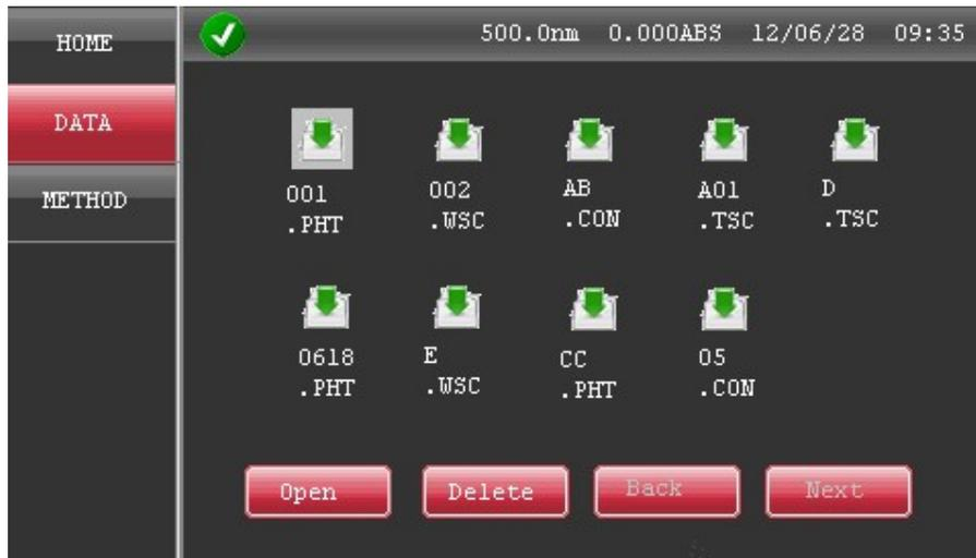
This interface is used to manage all method data document. Open or delete the measure data document . Each page displays 10 data document. Using this function, the user must load SD card. Measure data is saved in SD card.
