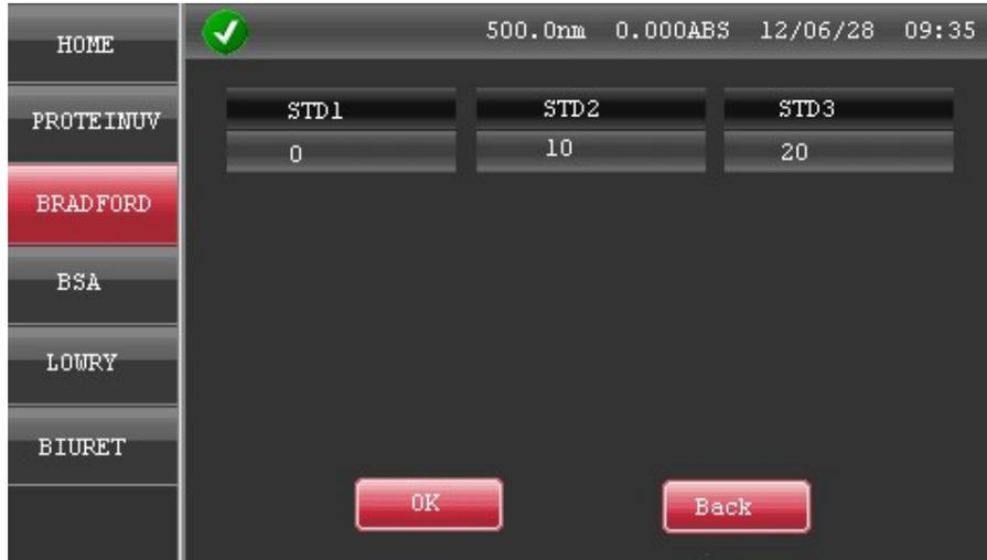
STD1~3 standard sample concentration setting (According to the number of concentration in the upper layer interface, it will display corresponding setting)
