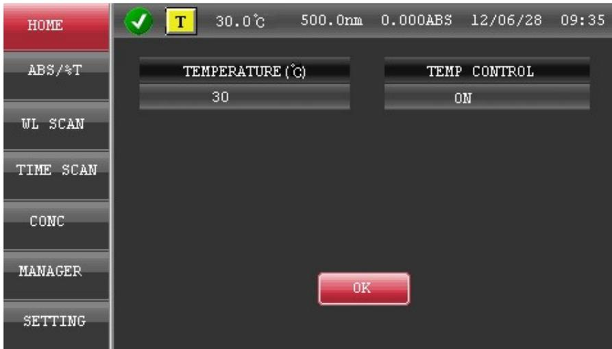
TEMPERATURE (°C )    setting control temperature
