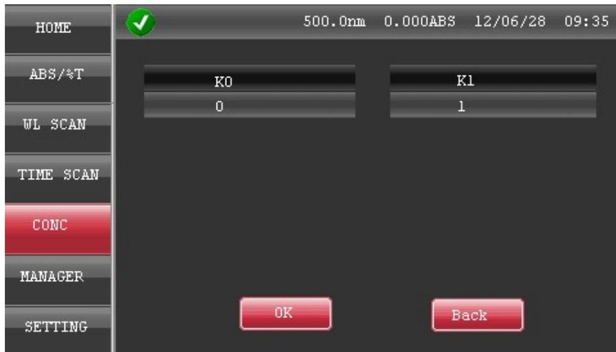
If using regression equation parameters to enter calculation method ( CALIBRATION, select K-Factor ) ,it will show this parameter setting interface.
