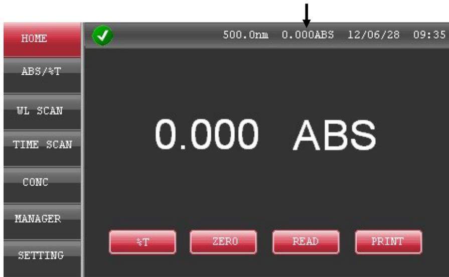
This interface is used to measure single wavelength's absorbance or transmission. In any interface (non-execution of measure in the interface), click value in the status bar into the large character measure.
