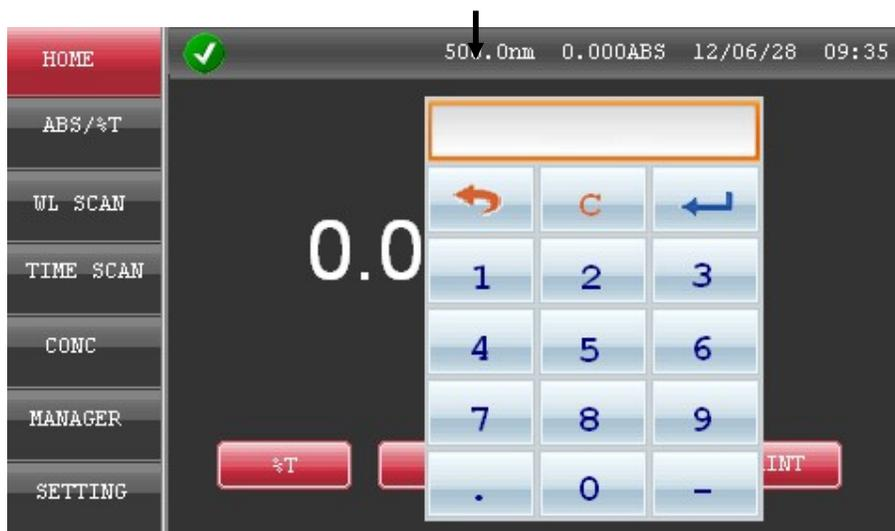
In any interface (non-execution of measure in the interface), click wavelength in the status bar, input wavelength, the instrument will move to the target wavelength. (GOTO  $\lambda$  function)
