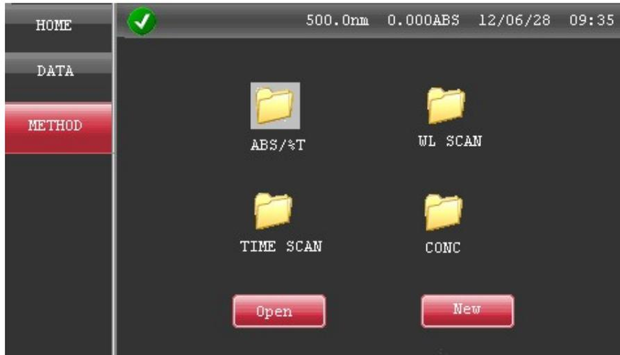
This interface is used to manage sample measure methods. User can select and save measure methods. Preview and open previous measure methods. Use this function, user must load SD card. Measure methods and measure results document are saved in SD card.
