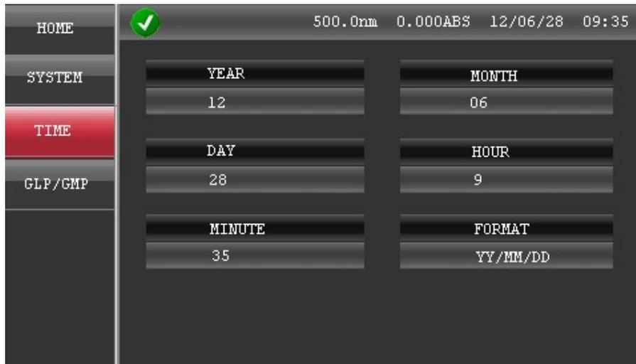
This interface is used to set up time. The instrument has power-down protection capacity (in general, about 96 hours). Switching off the instrument for 96 hours, the user need to reset time, but the setting data will be not lost.
