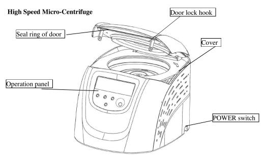
Figure 5.1 Front view of centrifuge
