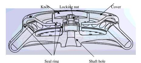
Figure 11-1 The rotor structure
