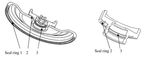
Figure 9-1 Seal rings of rotor
