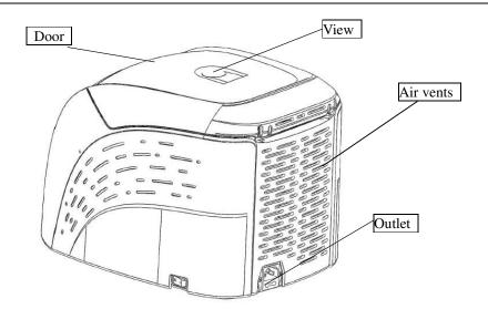
Figure 5.2 Rear view of centrifuge
