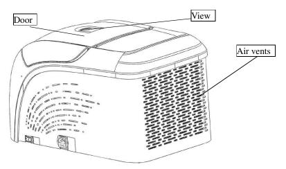
Figure 5.4 Rear view of centrifuge
