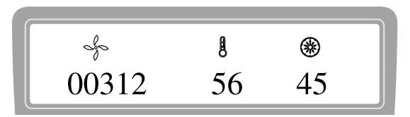
Figure 8-2 Accumulative running time interface
