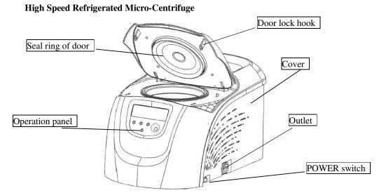
Figure 5.3 Front view of centrifuge
