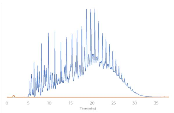
Fig 3. Overlay of Reference Gas Oil Sample with CS<sub>2</sub> Blank
