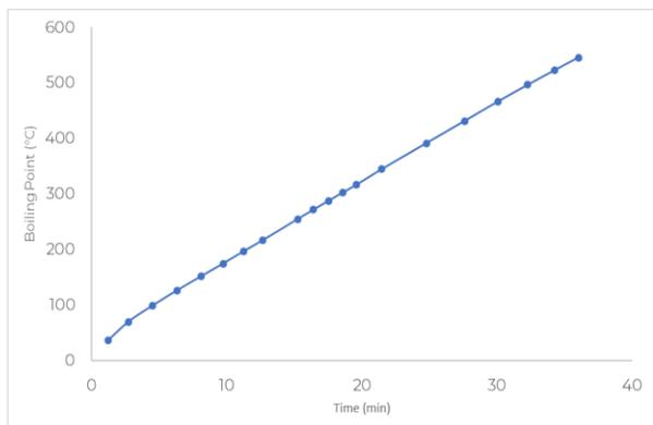
Fig 2. C5-C44 n-Paraffins RT vs Boiling Point Calibration
