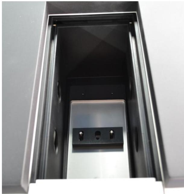
Figure 4-3 Removal of cuvette holder
