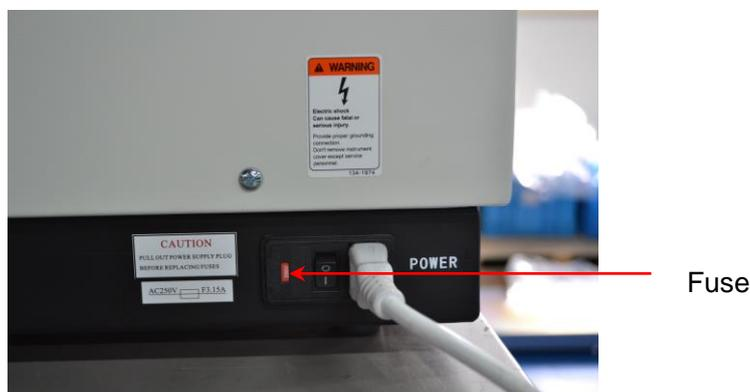
Figure 1-3 Power supply of UV2600 Spectrophotometer
