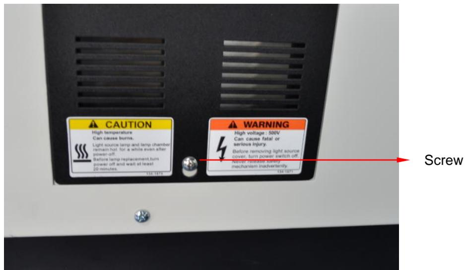
Figure 4-9 Removal of light source compartment cover
