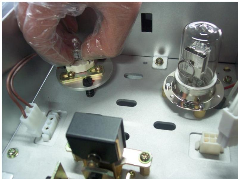
Figure 4-11 Removing WI lamp
